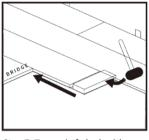
Step 7: Tap end of plank with hammer and tapping block to lock ends of planks together. Remove support bridge and continue with this method until you have completed installing the row.
